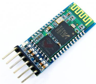
Gambar 3. Modul Bluetooth HC-05
