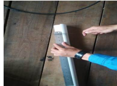
Gambar 3. Diameter pipa pvc 2 inci
