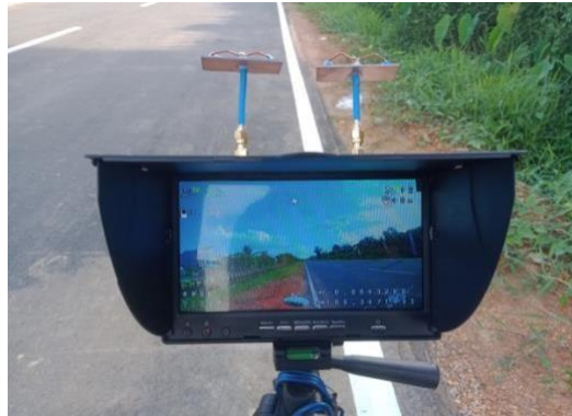
Figure 2. Directional biquad antenna on the monitor screen
