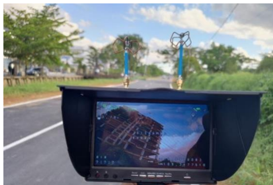
Figure 3. omnidirectional biquad 4 lobes antenna on the monitor screen
