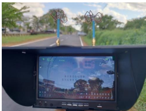
Figure 4. Omnidirectional biquad 6 lobes antenna on the monitor screen
