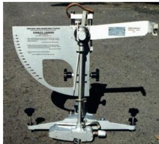
Gambar 1. Alat uji BPT (*British Pendulum Tester*)
