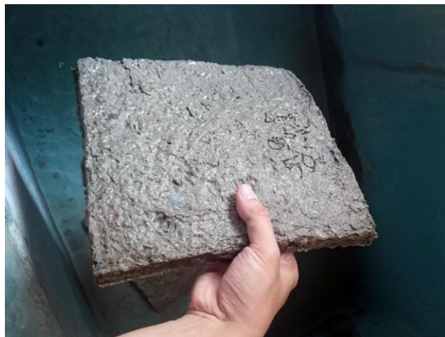
Figure 3. Bending on 1 cm Thickness Recycled Paper Panel without Cement Layer Source: Author's Documentation, 2016
