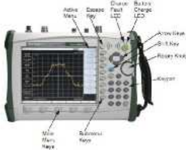
Gambar 1. Panel depan Spectrum Analyzer (SPA) merk Anritsu MS2665C
