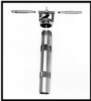
Gambar 4. Alat pengambil sampel sedimen (<http://www.rickly.com/as/images/HANDCOR E.JPG>)
