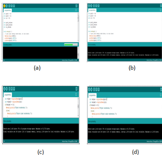
Gambar 10. (a) Proses Verify (b) Proses Verify Berhasil (c) Proses Upload (d) Proses Upload Berhasil
