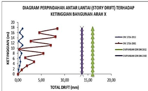
Gambar 11 Diagram Story Drift arah X
